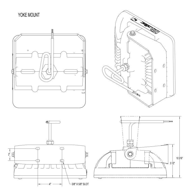
Securely tighten yoke mount fasteners when desired fixture orientation is achieved.
