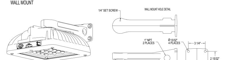
Securely tighten set screws when desired fixture orientation is achieved and the conduit connection is tight.
